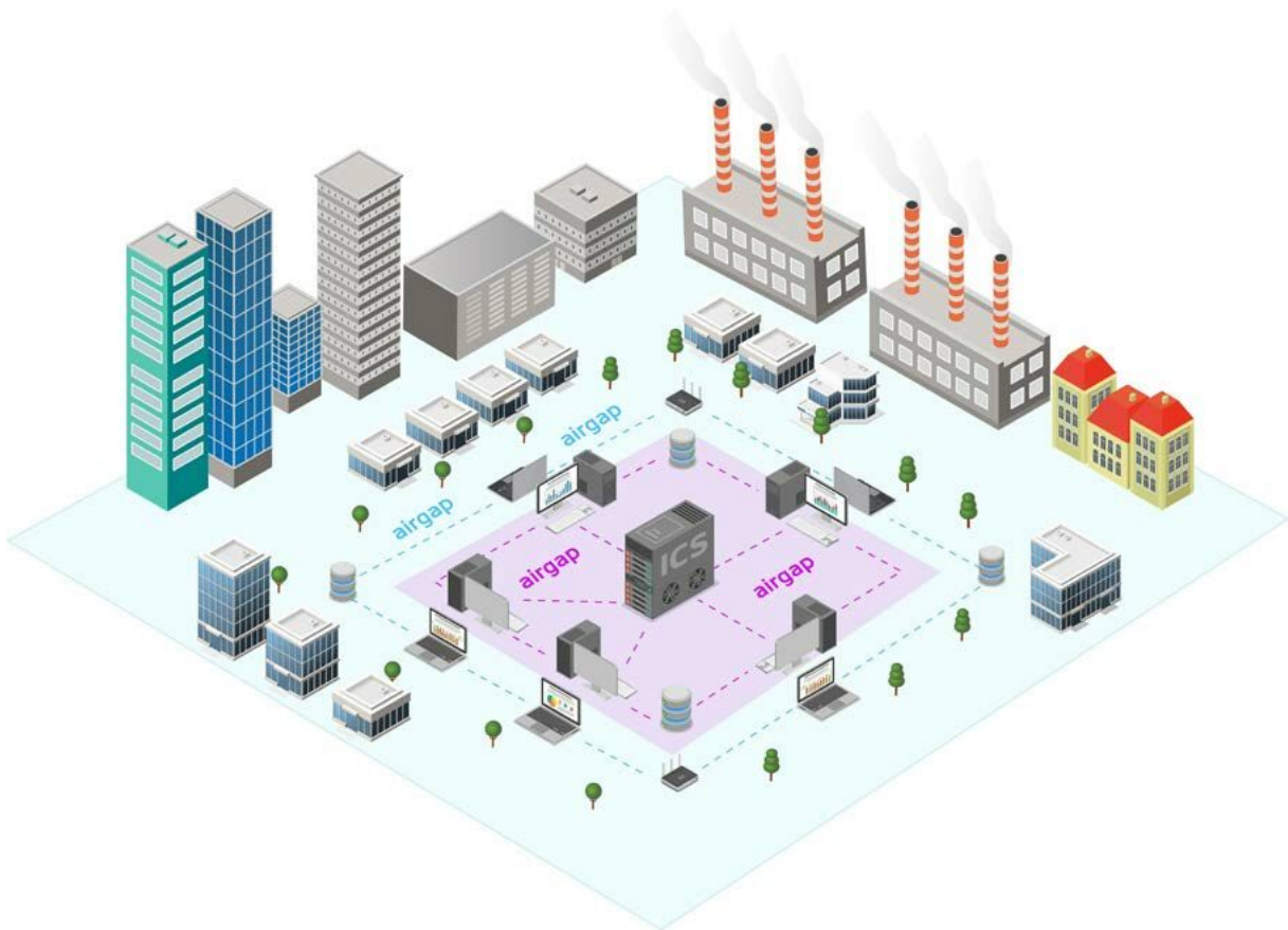
Figure 12: Isolated network from external network
