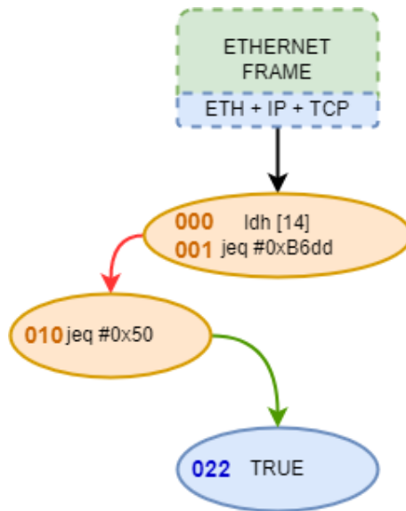
Fig. 2.6. Shortest path in the CFG described in the example of figure 2.5 that a packet needs to follow to be accepted by the BPF filter set with tcpdump .
